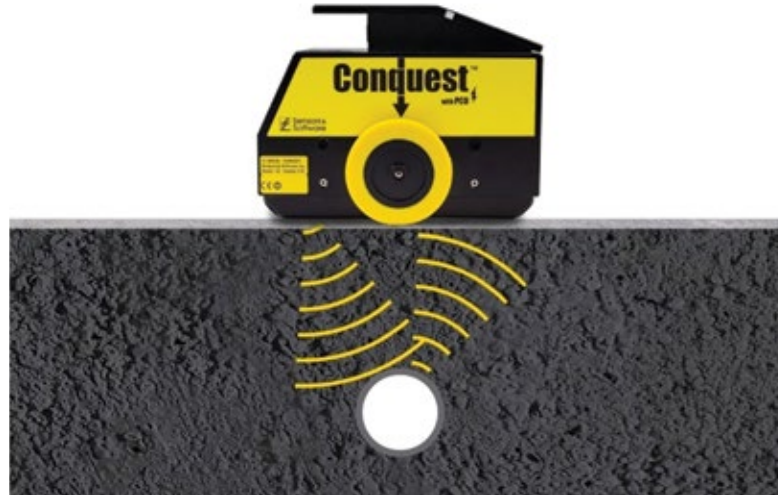
Figure 1: GPR measures the travel time for the transmitted wave, to and from an object in the concrete.
